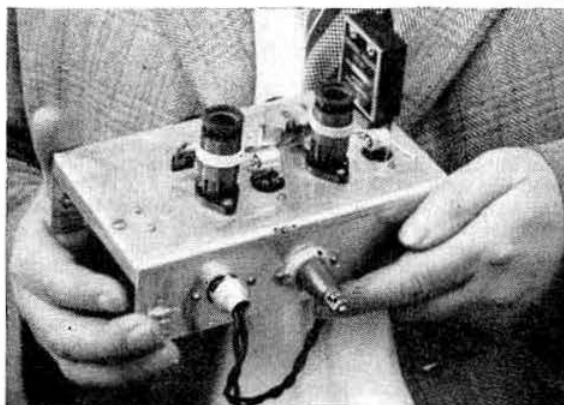
Here is a picture of the transistor transmitter used by G3CCA of Leicester. The p.a. coil is to the left followed by a GET1. The v.f.o. coil and a GET 2 are on the right. The crystal (1850 kc/s), used for netting, is in the right-hand top corner. Outstanding contacts have been with GM3EFS (275 miles) and G2FP (170 miles).
